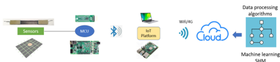
Figure 7: General concept of the wireless sensor network.
