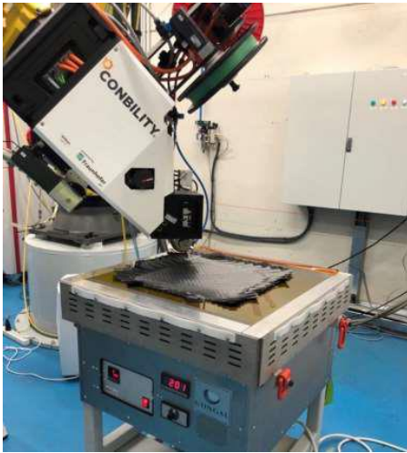
Figure 2: AFP machine with heated table and online pyrometers at AIMEN Technology Center
