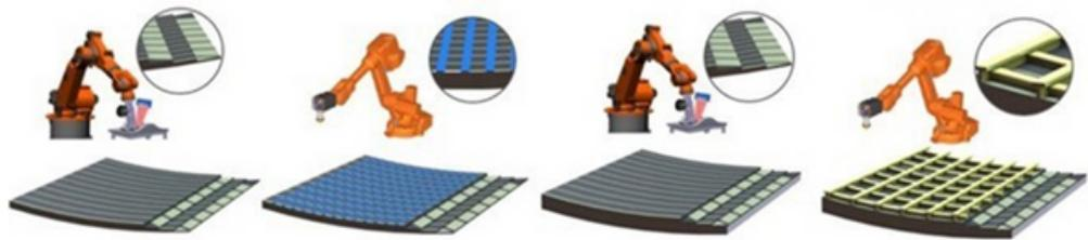
*Figure 1: Fabrication scheme combining AFP and FFF of the DOMMINIO demo*
