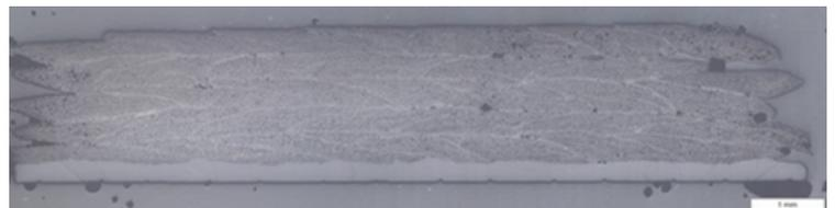
**Figure 11:** Cross section of a ILSS sample
