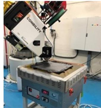
**Figure 5:** laminate being consolidated on a heated layup tool
