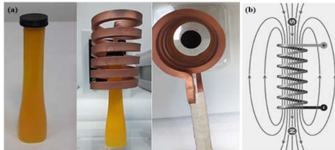
Figure 2. (a) Sample holder and solenoid coil for induction-heating testing and (b) electromagnetic field produced in solenoid coil (right).
